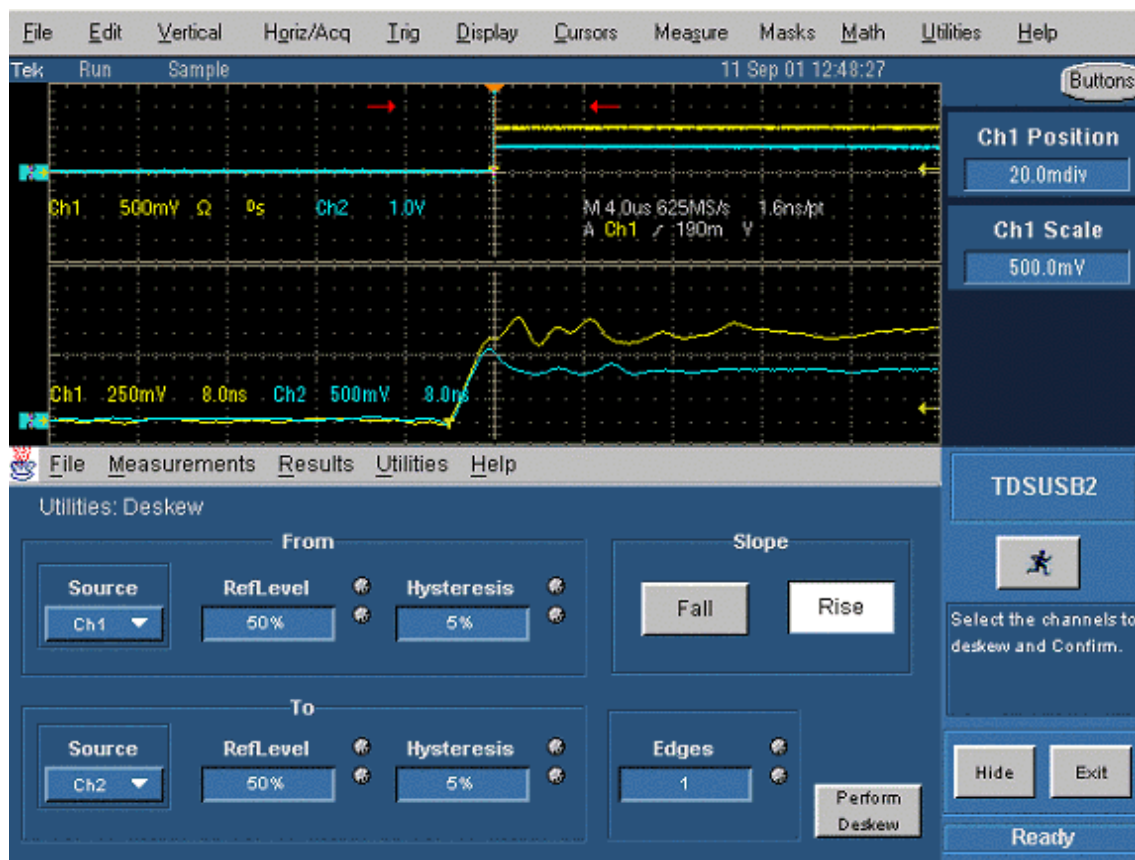
Figure 2: Signals after deskew
