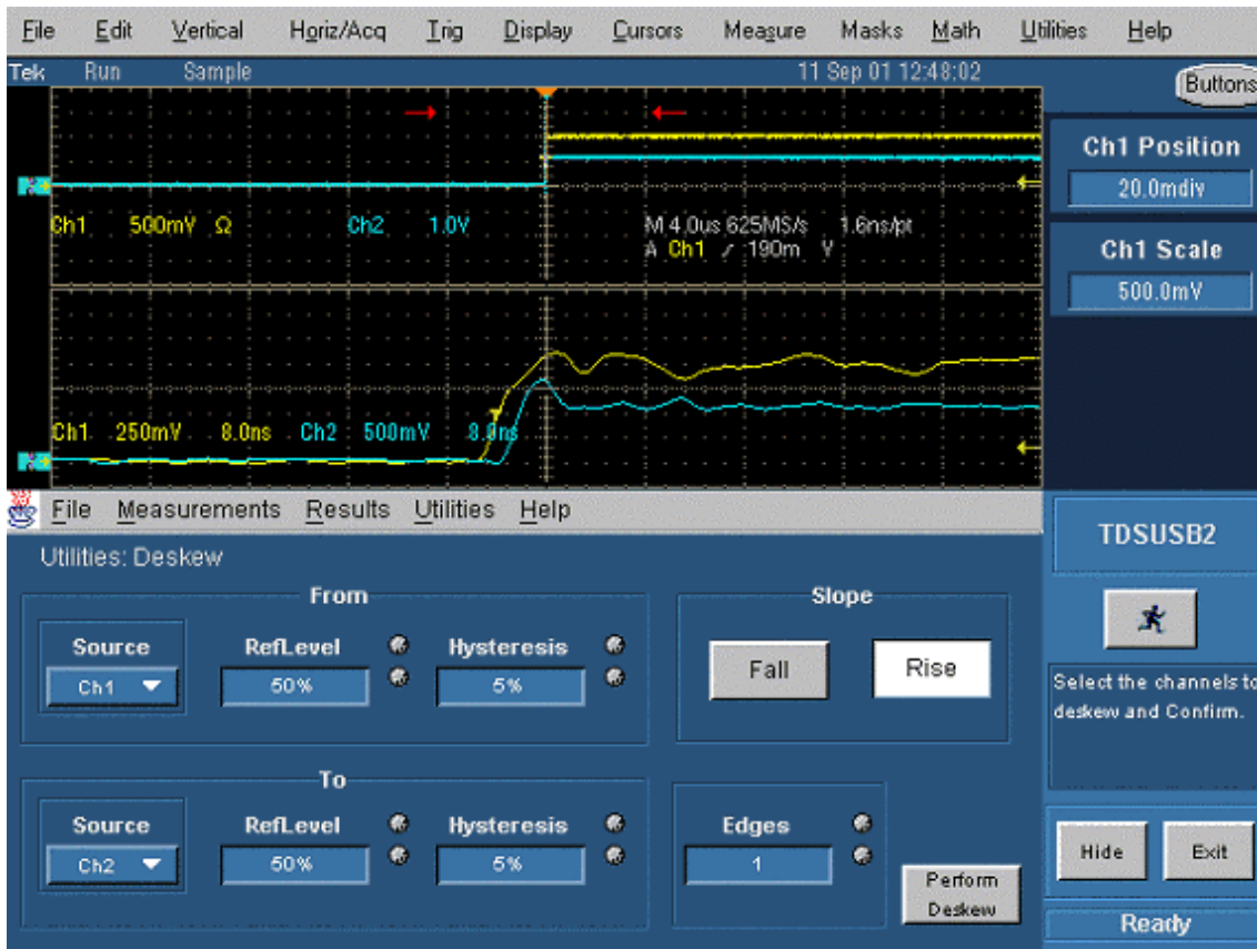
Figure 1: Signals before deskew
